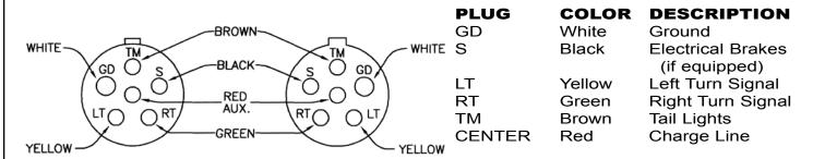
NOTE: Identify contacts by looking into the open end of plug or socket.
