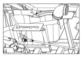
Before operating the vehicle, check the shift lever as to change gearshift from 1 to 5 and reverse smoothly.
