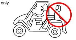
The total weight of operator, passenger, accessories, cargo, trailer tongue weight, and the vehicle itself must not exceed 845kg (1861lb). Carrying a passenger and cargo can affect vehicle handling.
