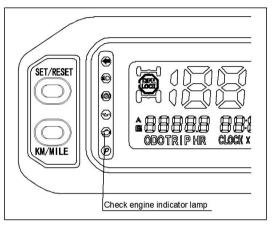
After turning the ignition switch on, the lamp shall be on, and the lamp shall be off after starting the engine. If the light is on while the engine is on, it indicates that the system has an error.
