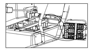
To install a seat, insert the fittings on the rear of the seat into the holders and push down on the seat at the front.
